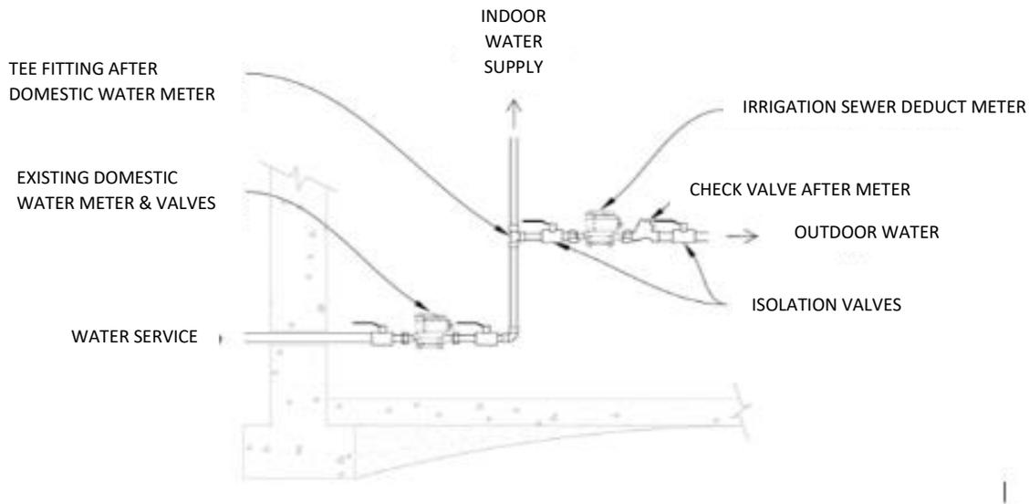
A cross-connection occurs whenever the drinking water supply is or could be in contact with potential sources of pollution or contamination. Cross-connections exist in piping arrangements or equipment that allows the drinking water to come in contact with a pollutant in the event of a backflow.
